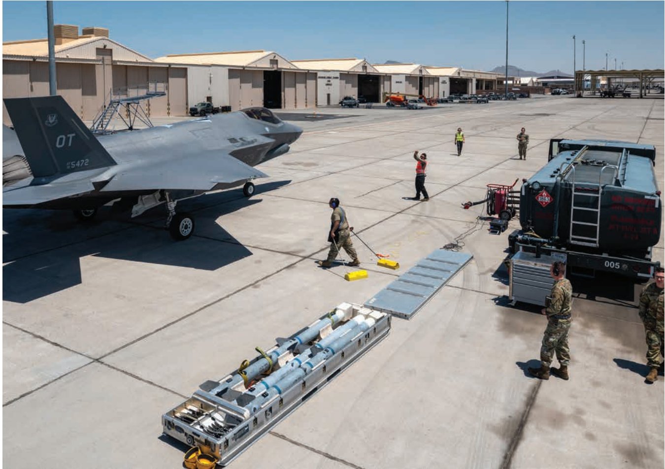
U.S. Airmen at Nellis Air Force Base test newly approved F-35A hot integrated combat turn procedures, focusing on safety, efficiency, and physical demands, 23 Jun 25. With support from the 57th Maintenance Group, teams from the 59th Test and Evaluation Squadron and Human Performance Office use a hybrid loading method and monitor physiological impacts to help shape future tactics. Photo by William R. Lewis
